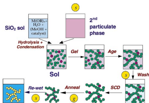
Fig. 4 Points during sol-gel chemistry and processing at which the sol, wet gel, supercritically dried gel (aerogel), or re-wetted aerogel may be chemically modified; s = solution, g = gas phase.
